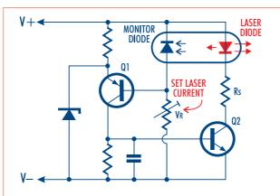
Fig.7: How the monitor diode is used to control the laser operating current and optical output, in a simple feedback circuit.
