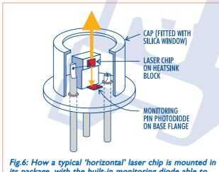
its package, with the built-in monitoring diode able to sense its 'rear' output... to increase with current level. So short pulses of significantly higher output separated by periods of no output actually result in a higher average light output, for the same average *current*.
