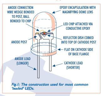
diameter 'bullet' type with a spherical front lens are the most common. Other much smaller packages are used for surface-mount LEDs, including 'naked' LED chips.
